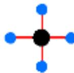
Figure 3 - Schematic of SSP&A method velocity calculation
