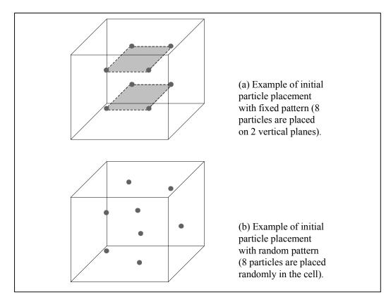
Figure 18. Initial placement of moving particles
