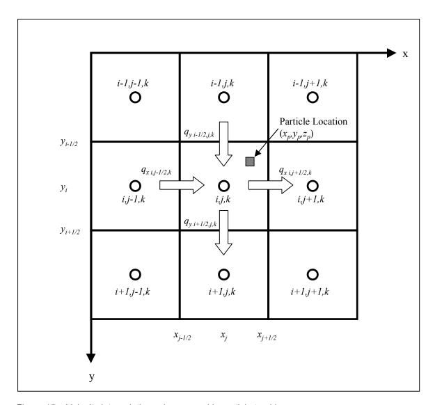
Figure 15. Velocity interpolation scheme used in particle tracking
