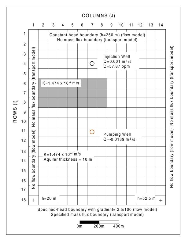
Figure 43. Configuration of the test problem involving transport in a heterogeneous aquifer with a strong regional gradient
