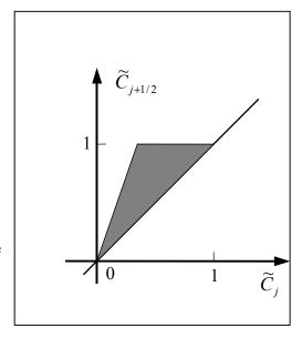
Figure 5. Illustration of the universal limiter constraints used in the ULTIMATE scheme
