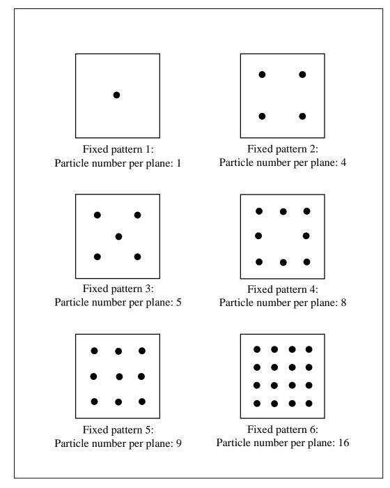
Figure 30. Distribution of initial particles using the fixed pattern (if the fixed pattern is chosen, the number of particles placed per cell (NPL or NPH) is divided by the number of vertical "planes," or NPLANE, to yield the number of particles to be placed on each vertical plane, which is then rounded to one of the values shown here)
