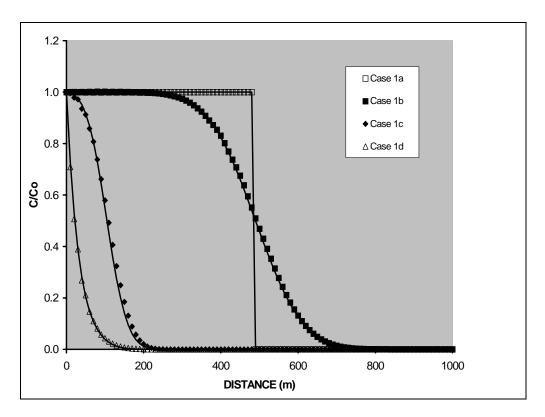
Figure 31. Comparison of the calculated concentrations with the analytical solutions (solid lines) and numerical solutions (symbols) for the one-dimensional test problem
