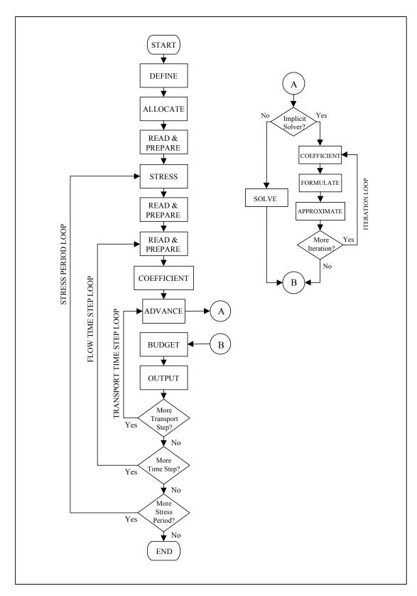
Figure 22. General procedures for a typical transport simulation
