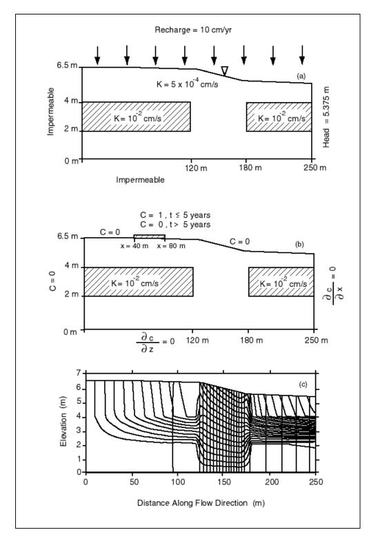
Figure 40. Physical system and flow boundary conditions (a), transport boundary conditions (b); and hydraulic head and stream function solutions (c) (contour intervals are 0.05 m for the hydraulic head and 1 m²/day for the stream function (Sudicky 1989))
