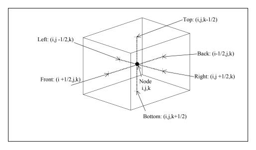
Figure 14. Definition of six surrounding interfaces of cell (i, j, k)
