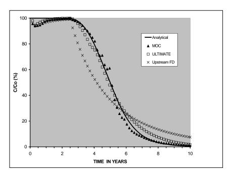
Figure 38. Calculated concentrations at an injection/pumping well as compared with the analytical solution of Gelhar and Collins (1971)
