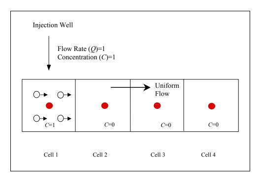
Figure 21. Illustration of the mass balance problem associated with an Eulerian-Lagrangian technique due to the discrete nature of moving particle methods
