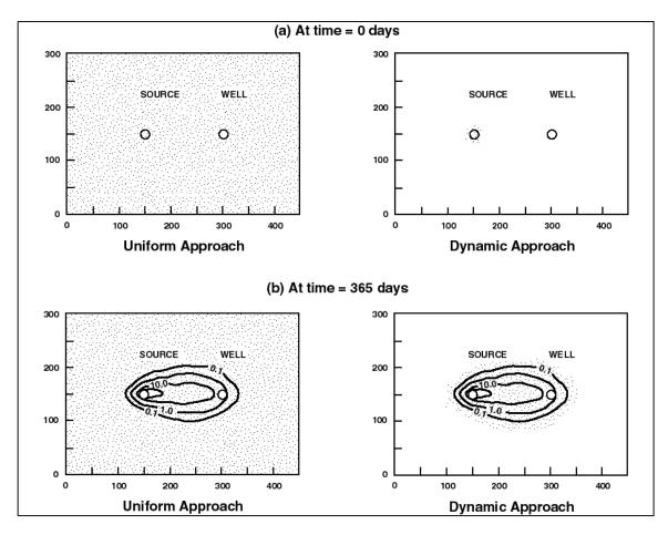
Figure 17. Comparison of the uniform and dynamic approaches in controlling the distribution of moving particles
