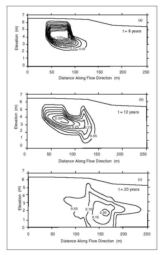
Figure 41. Plume configuration at (a) t = 8 years, (b) t = 12 years, and (c) t = 20 years based on the LTG method from Sudicky (1989)
