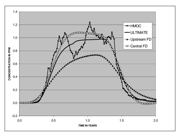
Figure 45. Comparison of the calculated concentration breakthrough curves based on different solution schemes at the pumping well
