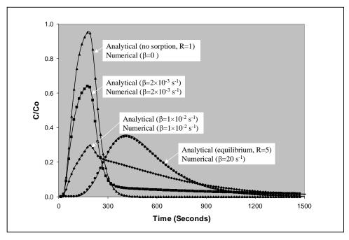
Figure 34. Comparison between the analytical solutions (solid lines) and numerical solutions (symbols) for one-dimensional transport involving nonequilibrium sorption
