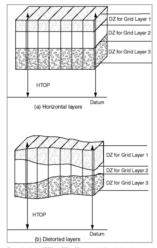
Figure 28. Arrays HTOP and DZ for different vertical discretization schemes
