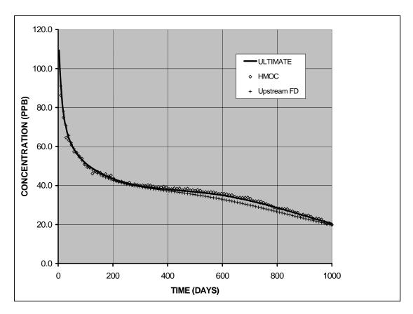
Figure 50. Concentration breakthrough curves as calculated using different solution schemes at the pumping well W4, located near the middle of the initial plume
