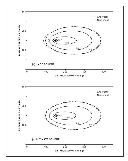
Figure 35. Comparison of the analytical and numerical solutions for twodimensional transport from a continuous point source with the model grid aligned with the flow direction
